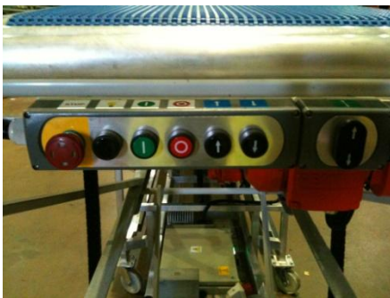
...the Command unit for all control commands and emergency-stop
