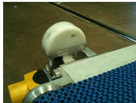
...photo-cells at each end-position stop the conveyor once the goods are not unloaded timely ....
