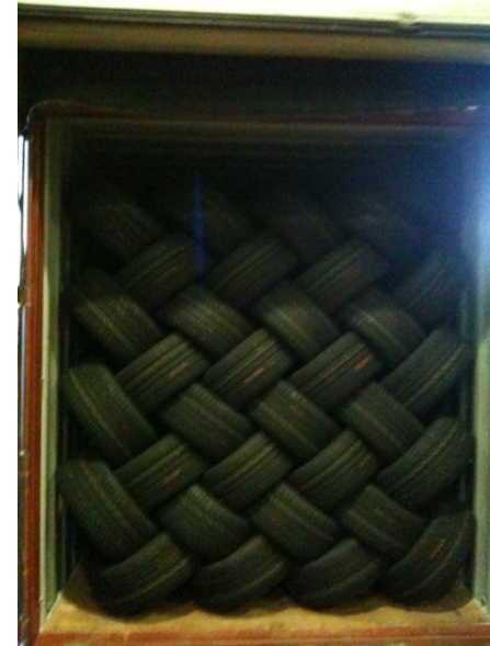
Example for a loading with the conveyors and the utilisation of the complete height inside
