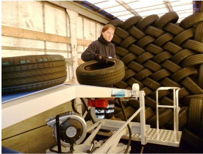
...for best ergonomic working conditions the platform is lifted level by level either downwards....
