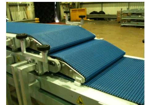
...the special designed ramps allow a tyre transport in each direction....
